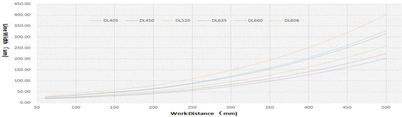
Adjust the focus at different WD and test the line width_ J006
